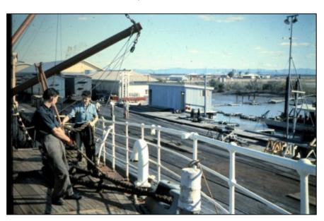
The tidal range in Port Alma was large so the mooring ropes needed adjusting frequently, in this shot two midshipmen are adjusting the mooring ropes so that the ship does not get 'hung up' on the wharf or drift off it.
